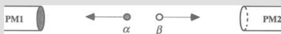
FIGURE 5.8. Two correlated photons \alpha and \beta enter the photodetectors PM1 and PM2 , respectively.
